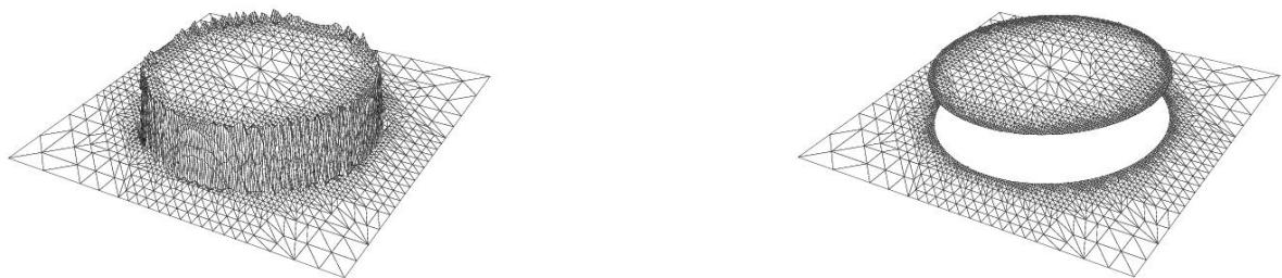
Figure 1: Pressure jump of a static bubble using piecewise linear FEM (left) and suitable XFEM (right).
